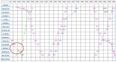
Figure 4. A snapshot of the re-schedule timetable in scenario 3, where the trajectory of iron ore train 19911 through station Björkliden is not optimal from an eco-driving perspective.
