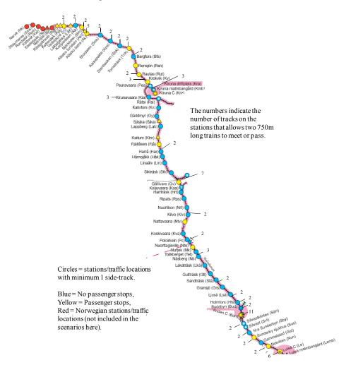
Figure 2. Overview of the studied railway line Björnfjell-Riksgränsen-Kiruna-Boden-Luleå and its characteristics. The stations indicated with a number, are stations that can accommodate two long (750m) freight trains and the number specifies the number of tracks. Source: Compilation of illustrations and data provided by Trafikverket.
