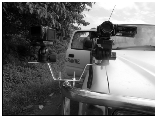
Figure 3-3: Cameras clamped on the vehicle guard rail
